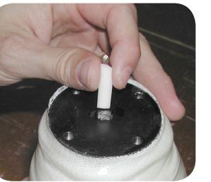
Press the Proximal Gasket into the pump inlet.
