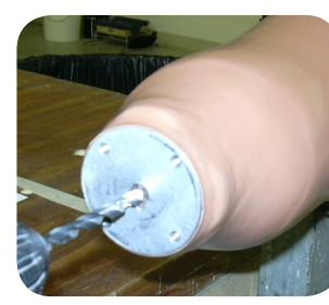
Remove the model. Trim as desired. Drill a 9/32" diameter hole in the socket.
