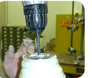
Push the filter into the hole. Cut it flush with the the socket.
