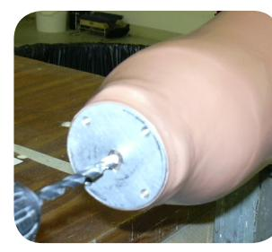
Push the filter into the hole. Cut it flush with the socket.
