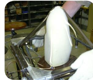
Rough up the surface of the PETG. Clean with rubbing alcohol (do NOT use acetone).
