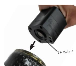
*Note: you should be able to turn the pump upside down without the gasket falling off. If the gasket falls off, it was not properly seated into the recess.*
