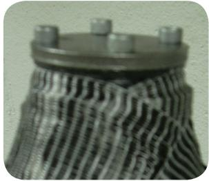
Apply the layup. Tie off in the space between the forming plate and 4-hole Adapter. Pull the rest of the layup down. Laminate.
